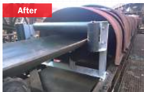
The hold-down roller and guide roller functions prevent belt lift-off and mistracking, ensuring stable operation.
